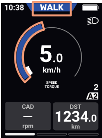
Walk assist mode (assistance functioning)
